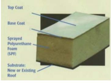
For each inch of foam added to your roof you gain an "R" factor of seven to the roofs insulation.
