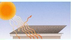
An uncoated roof can absorb up to 83% of the sun's heat and UV rays.
