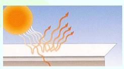
A roof coated with a White Roof Coating can reflect up to 88% of the sun's heat and UV rays.
